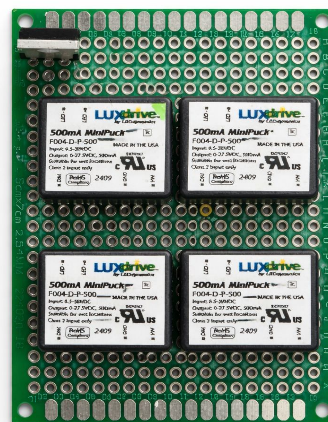
Figure 4. Resoldered MiniPucks and Mosfet.
